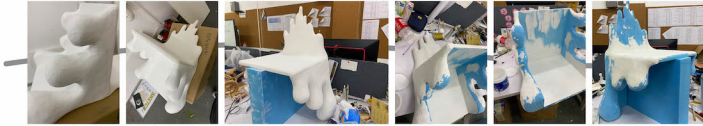
I used high-density foam, putty to create the base appearance of the model and sandpaper to smooth it out.
